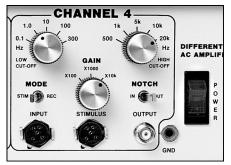
the **INPUT** connector is connected to the signal from the **STIMULUS** connector and the **OUTPUT** connector is disabled. In Record Mode, the **INPUT** connector is connected to the amplification circuits and the signal is available at the **OUTPUT** connector.
