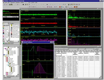
**EMG and EEG** - The example experiment is configured to continuously record both EEG and EMG. Simultaneously bursts of EMG activity are detected using the Experimenter burst analysis. The burst durations and inter burst intervals are calculated and counted with the values automatically displayed in the realtime spreadsheet.
