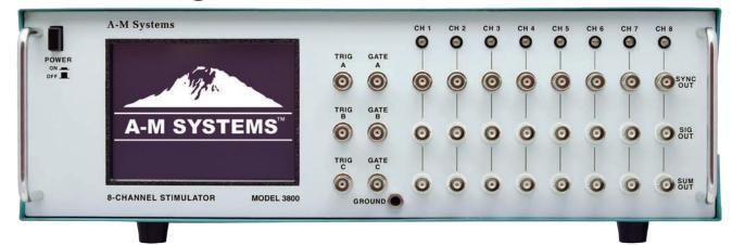
*The Model 3800 MultiStim 8-Channel Programmable Stimulator* is a multichannel programmable stimulator designed for a wide variety of applications. It is highly flexible, being capable of simultaneously delivering up to eight different series of pulse trains comprised of monophasic or biphasic pulses. In addition, the unit can produce trains of stepped pulses or paired pulses with easy to use built-in protocols.
